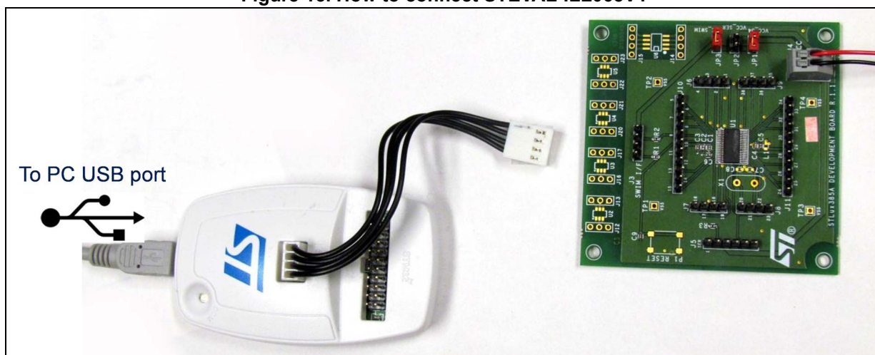
Figure 15. How to connect STEVAL-ILL068V1
