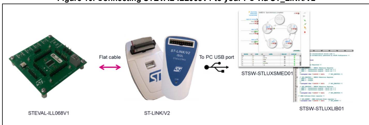
Figure 10. Connecting STEVAL-ILL068V1 to your PC via ST_LINK/V2
