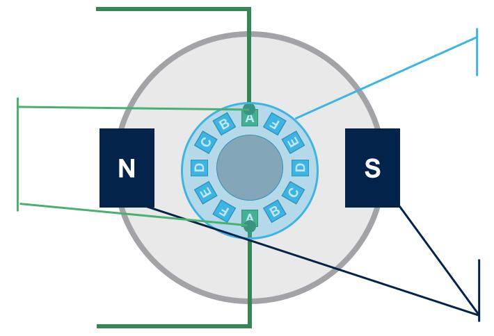
The rotor is composed by a group of coils
