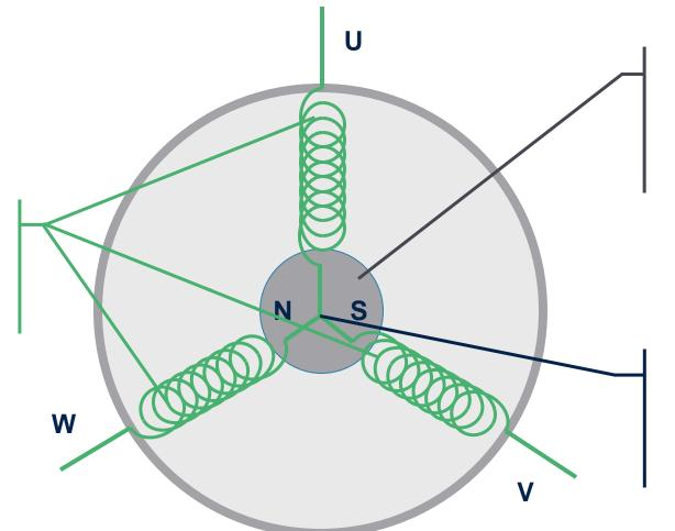
A permanent magnet generates the magnetic field of the rotor
