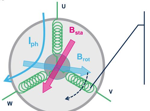
When the magnetic field of the rotor crosses the unloaded phase, the respective BEMF voltage changes polarity (zero-crossing)
