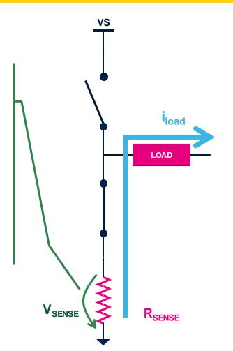
In some cases, the current doesn't flow into the shunt resistor even if the low side switch is on.
