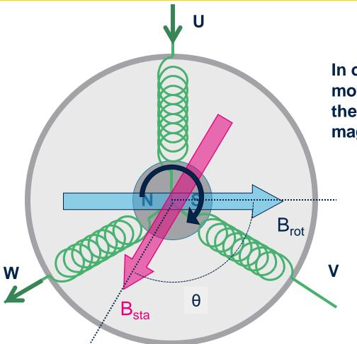
In order to keep the motor in motion it is necessary to change the direction of the stator magnetic field.
