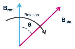
$$Tq \propto B_{rot} \cdot B_{sta} \cdot \sin(\theta) \propto I_{ph} \cdot \sin(\theta)$$
