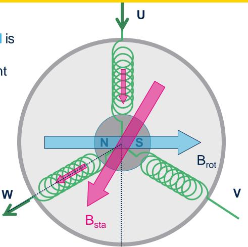
When a current flows from a motor phase to another one the magnetic fields are combined generating the stator field.
