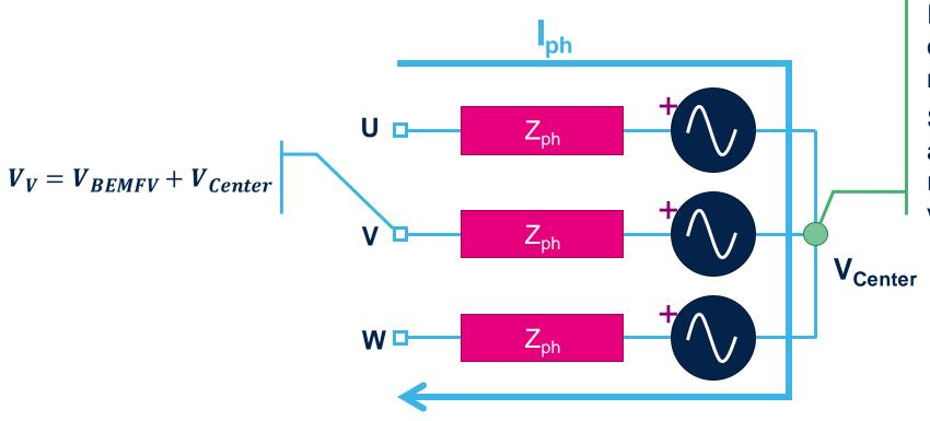
In order to detect the zero-crossing of the BEMF the center-tap voltage must be known.
