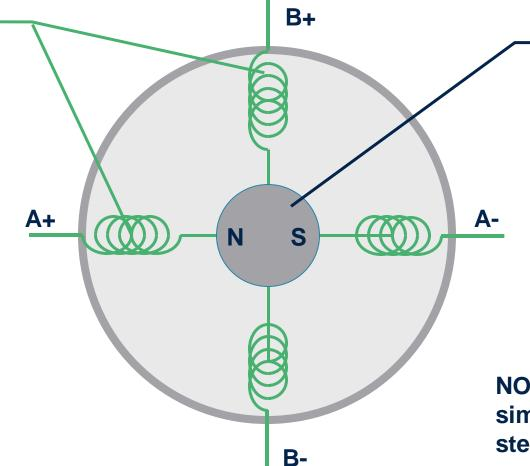
A permanent magnet generates the magnetic field of the rotor
