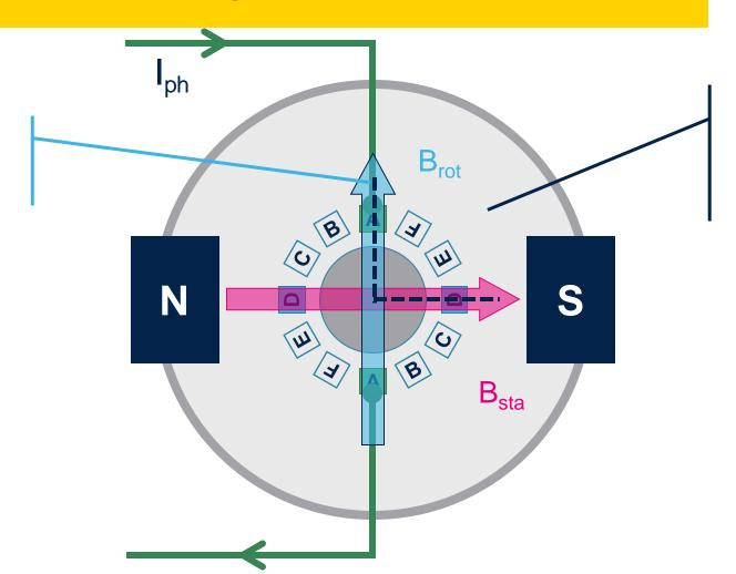
The torque applied to the rotor is the highest possible because the load angle  $(\theta)$  is about  $90^{\circ}$
