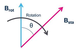
Usually one of the two is generated by a permanent magnet while the other one is generated through an electromagnet (solenoid).
