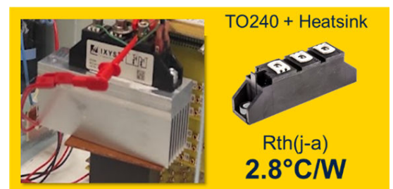
Figure 7. Junction to ambient thermal impedance
