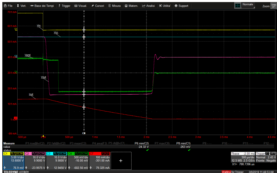
Figure 6. Measurement example ( T_{\text{DEMAG}} > t_{\text{D\_STBY}} ) with 4.7 kΩ GND resistor
