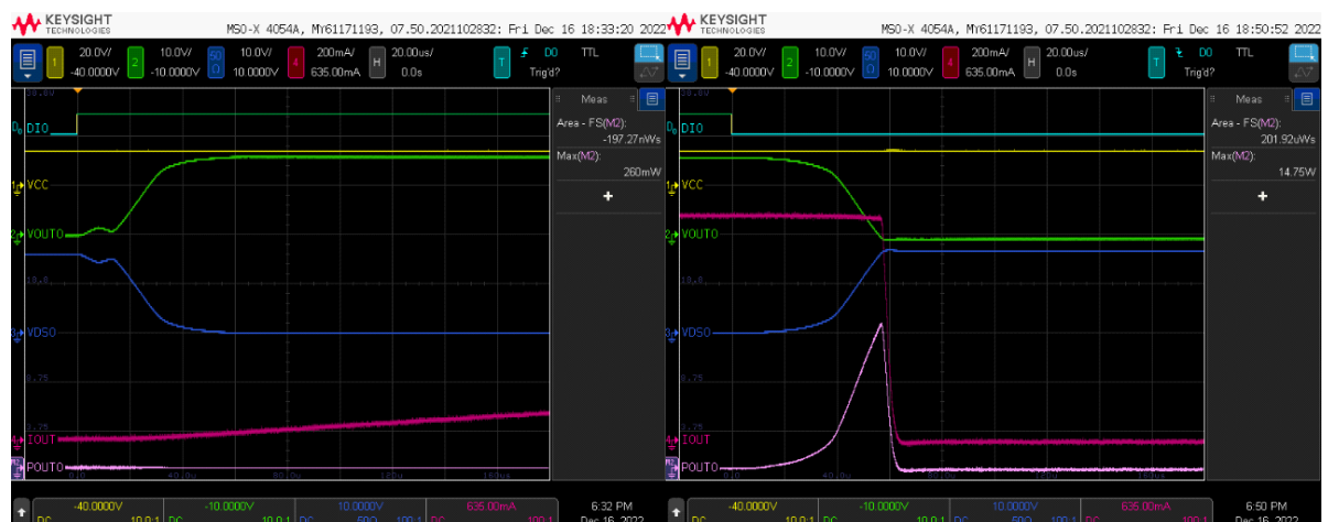
Figure 43. High inductance ( T_{\text{DEMAG}} > t_{\text{WOFF}} )–measurement example 1
