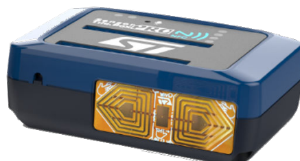
Figure 31. Qvar electrodes on the board
