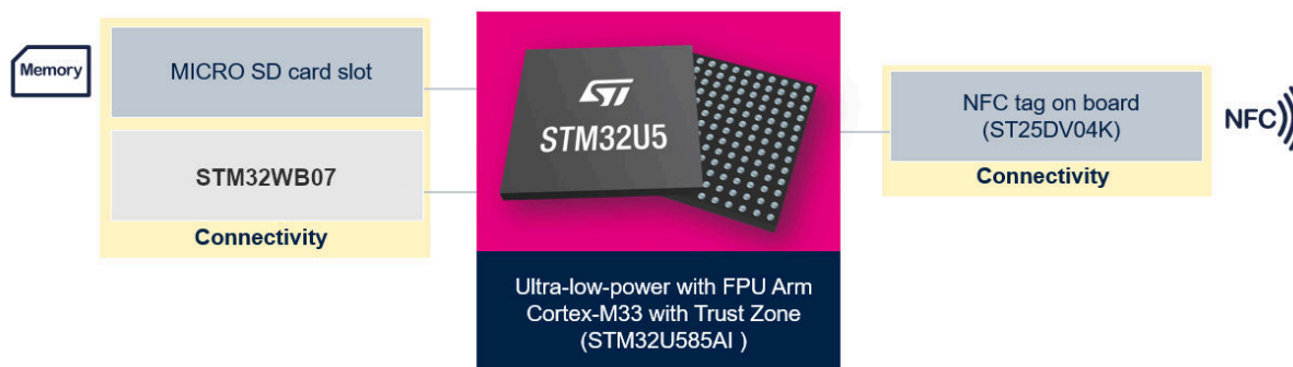
Figure 12. MCU and connectivity components (top view)
