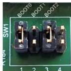
Figure 3. STM32MP135F-DK boot relay switch configurations
