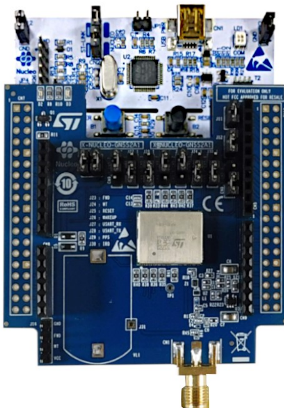
Figure 25. X-NUCLEO-GNSS2A1 expansion board connected to an STM32 Nucleo board
