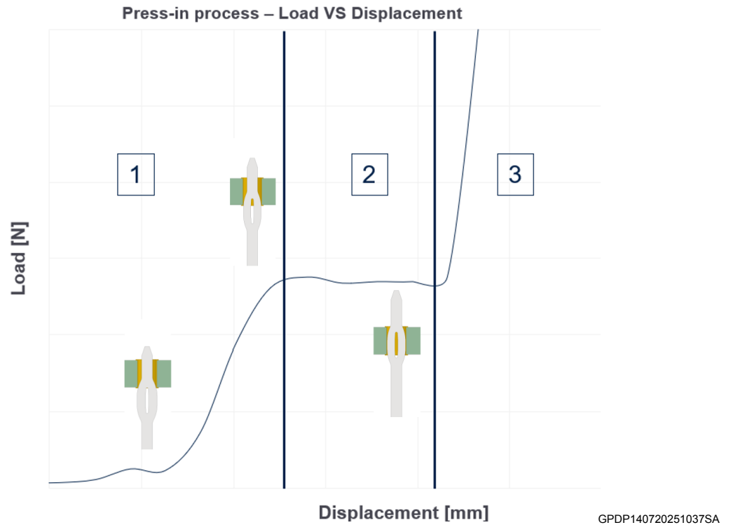
Figure 12. Typical press-in-force profile for insertion with distance keeper
