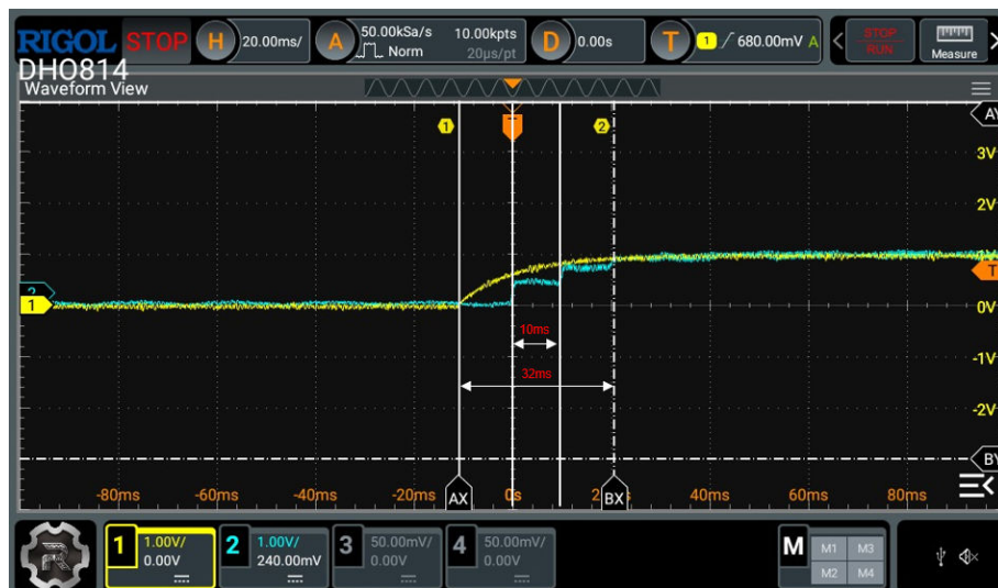
Figure 7. Input sense signal (yellow) vs output signal generated (blue) - Transition from 0 to 1 V
