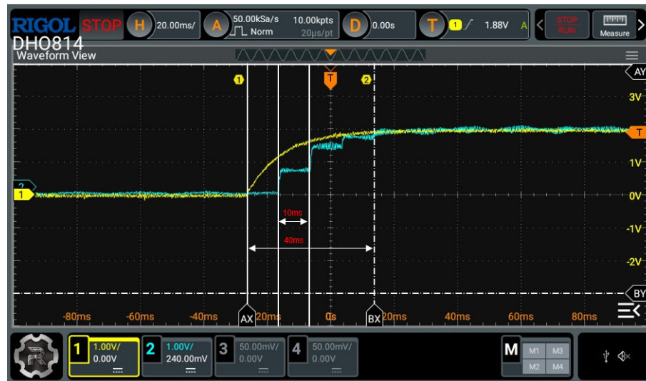
Figure 9. Input sense signal (yellow) vs output signal generated (blue) - Transition from 0 to 3.3 V
