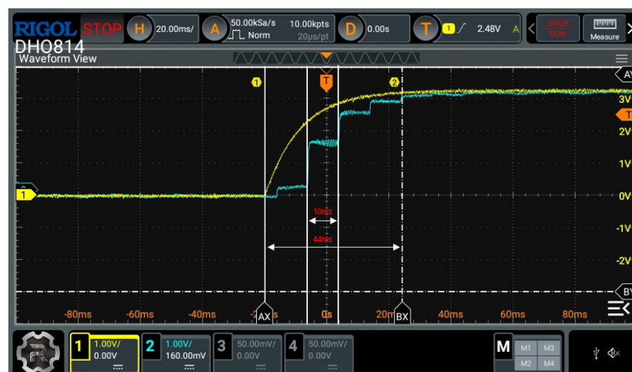
Figure 9. Input sense signal (yellow) vs output signal generated (blue) - Transition from 0 to 3.3 V
