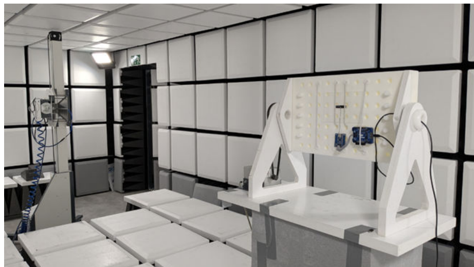
Figure 6. Anechoic chamber illustration
