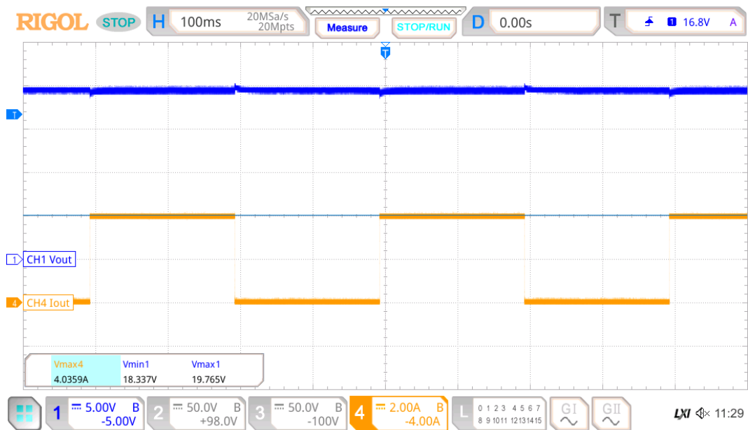
Figure 10. Dynamic step load - 90 Vac
