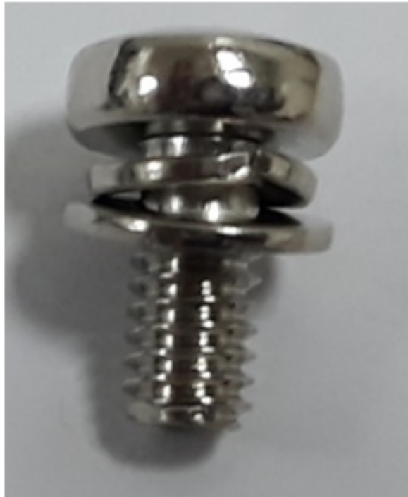
Figure 9. Example of SEMS Nickel plated screw size M4 x 0.7 with spring and plain washer
