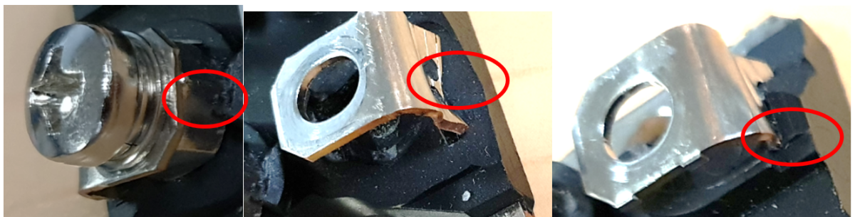
Figure 8. Pictures of resulting mechanical damage on ISOTOP package
