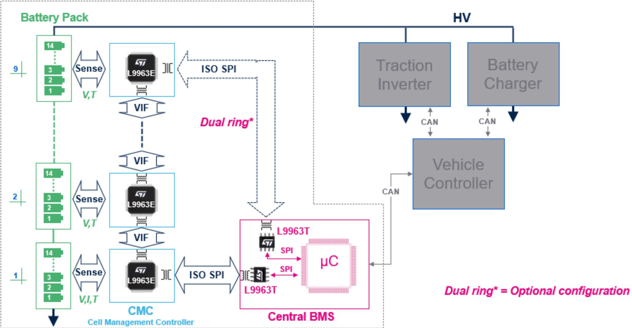
V,I,T = Voltage, Current and Temperature sense
