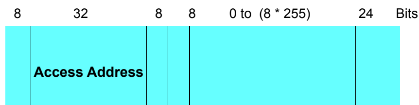
Figure 5. Packet structure with LE data packet length extension feature
