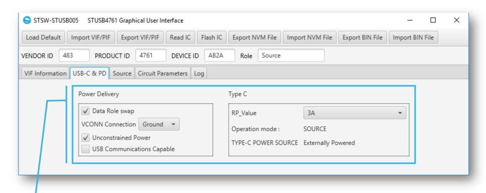
Configuration of STUSB4761 Type-C parameters and generic USB PD parameters.
