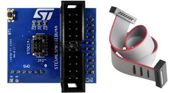
STEVAL-MKIGIBV4 + Cable STLINK Adapter (V2, V2.1)
