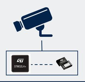
STSAFE-A is embedded into the object to authenticate, connected to local host MCU/MPU
