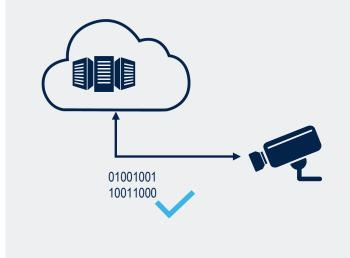
STSAFE-A ensures the integrity and confidentiality of exchanged data by ciphering and/or signing data
