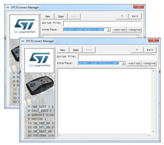
SPC5 Connect firmware is based on a script and an engine. SPC5 Connect explorer works only with the default firmware but the user can change the script to execute personalized tasks.
