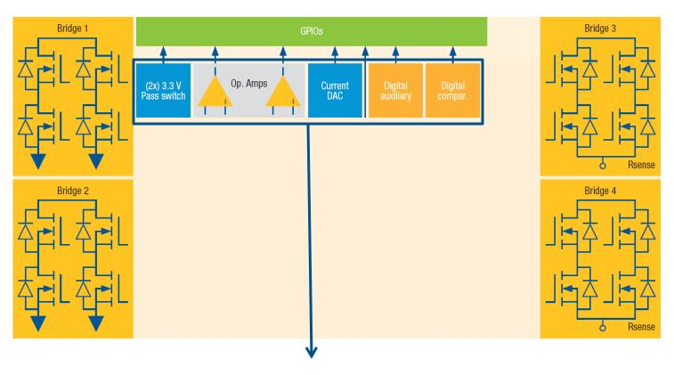
OpAmps, digital comparator, current DAC, pass switches can be *configured* defining gains, reference voltage, current levels etc..
