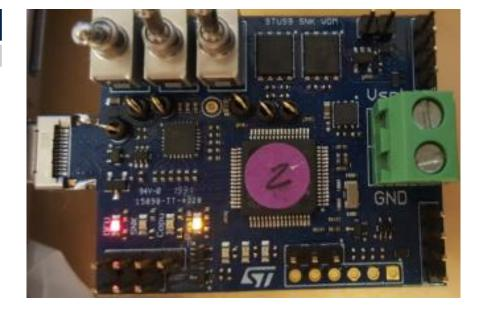
4 Check that Red and Orange LEDs are continuously ON
