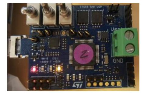
7 Check that Red and Orange LEDs are continuously ON
