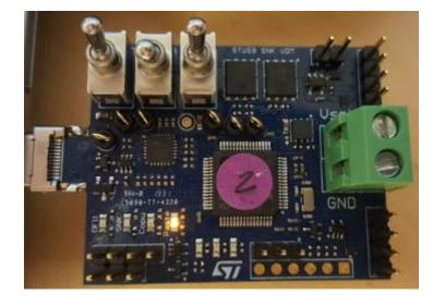
8 Ensure that Orange LED is continuously ON
