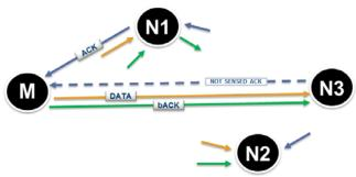
Figure 3: Data communication flow with a case of repetition.
