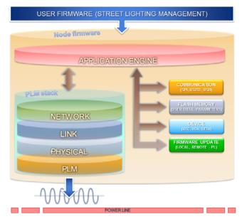
Figure 2: Firmware structure of the power line modem.
