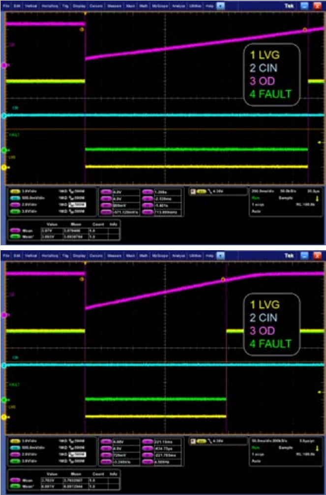
Figure 6: On the first figure C_{OD} = 2.2 \mu F , on the second figure C_{OD} = 330 nF .
