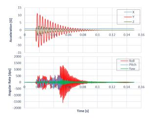
Figure 3: Mechanical response to a single step movement (Full Step resolution mode)
