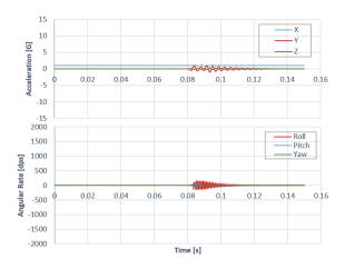
Figure 4: Mechanical response to a single step movement (1/256th Step resolution mode)
