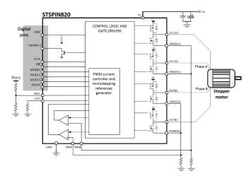
Figure 1: Block diagram of a typical application using the STSPIN820
