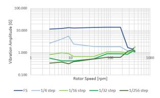
Figure 5: Vibration VS speed at different microstepping resolution
