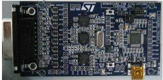
This family of boards is composed of two evaluation boards: the STEVAL-IME002V1 and the STEVAL-IME002V2 respectively designed to demonstrate the use of HM301D in Electrocardiographs (or patient monitor systems) (ECG) and Automated External Defibrillator (AED) configurations. They also host a 32-bit microcontroller of the STM32 family that manages the SPI protocol of HM301D and the USB communication from/to the PC. Any board could be easily used with dedicated PC
