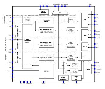
The ST HM301D (see Figure 4) provides a suitable solution for the ECG signal acquisition by offering, in addition to the above mandatory features, a series of fully integrated and configurable digital band-pass filters that allow selective analysis of the ECG wave by physicians.
