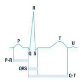
These ECG signals have diagnostically significant frequency content between 0.05 and 250 Hz. To ensure perfect acquisition of signals, the Analog Front End has to guarantee amplification of the ECG signals and rejection of nonbiological (e.g. powerline noise) as well as extraneous biological interferences (e.g. EMG), to include a differential amplifiers with high gains and an excellent common mode rejection (CMMR) capabilities in the range of 80 –
