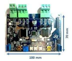
Figure 4: STEVAL-IHM042V1, Dual motor control board
