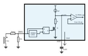
Figure 9 shows the injection of a small fraction of the line voltage into the bottom of the ILED capacitor. The small capacitor across the lower resistor is only to keep switching noise out of the circuit.
