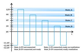
Fig. 2 IEC 61851 EV states with PWM signal
