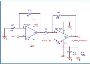
Figure 6: Measure conditioning stage.
