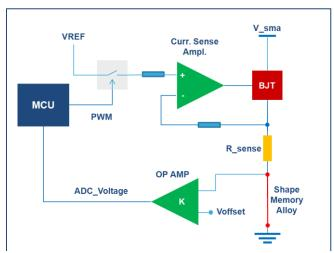
Figure 3: SMA current driver block scheme.
