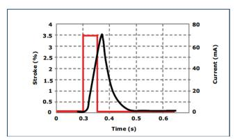
Figure 2. Stroke vs. Time [1st cycle, L=100mm, T=25°C, Max Curr.=70mA, Max Stress=170 MPa] (Courtesy of SAES Getters)
