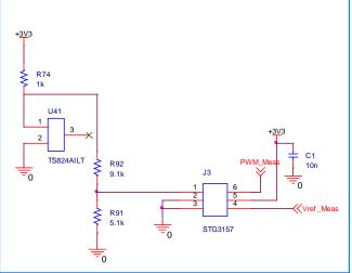
Figure 4: Current driver – control signal generator stage.
