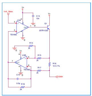
Figure 5: Current generator stage.
