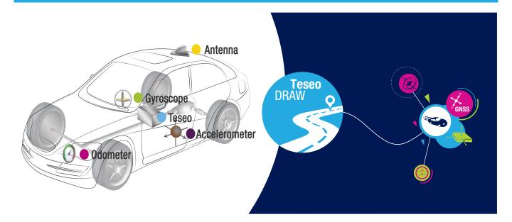
TESEO-DRAW firmware is a multisensor data fusion hub for ST's Teseo family of ICs. Thanks to filtering and predictive algorithms, TESEO-DRAW augments the user's positioning experience in terms of accuracy and availability, especially when the GNSS signal is degraded by environmental conditions (tunnels, urban canyons, indoor parking and multilevel highway junctions).
