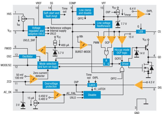
Built using ST's advanced BCD offline and BCD6 technologies, the L6566BH is an extremely versatile current-mode primary controller IC, specifically designed for high-performance offline flyback converters.
