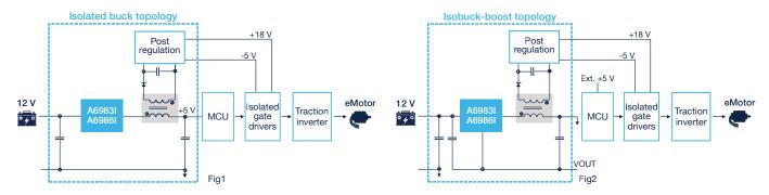
• Isobuck-boost topology: for each A6983I/A6986I device, this topology allows higher output power than buck topology to be delivered to the secondary side, and optimizes the transformer (figure 2). This topology can be evaluated through the STEVAL-A6986IV3, which is designed to supply 6 isolated gate drivers for a full three-phase inverter using a single A6986I device together with a 4-output transformer.
