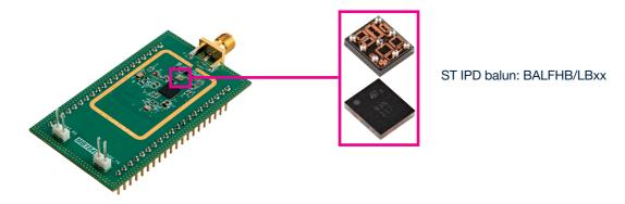
The baluns of STMicroelectronics integrate 3 functions: impedance matching, 50  $\Omega$  nominal input impedance and harmonic filter.
