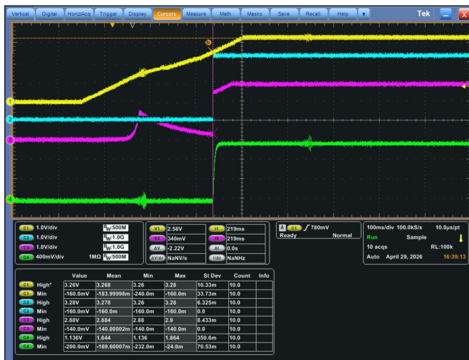
Figure 1. EN driven separately during VCC power-up (oscilloscope plot)
