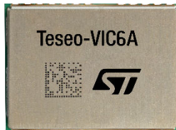
LCC 24 pins (16.0 mm x 12.2 mm x 2.42 mm)
