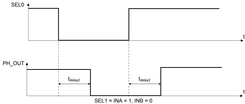
Figure 12. PH_OUT delay time on SELx change
