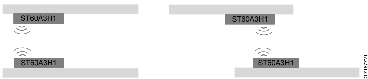
Figure 29. Supported ST60A3H1 180° relative orientations
