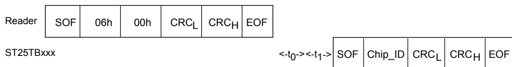
Figure 18. Initiate frame exchange between reader and ST25TB512-AT
