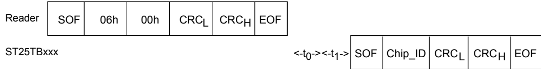
Figure 45. Initiate frame exchange between reader and ST25TB512-AT
