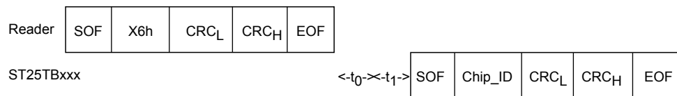
Figure 47. Slot_marker frame exchange between reader and ST25TB512-AT
