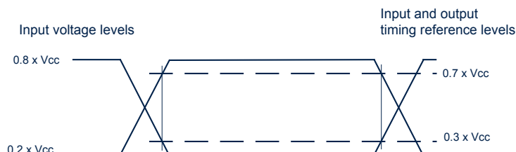
Figure 21. AC measurement I/O waveform
