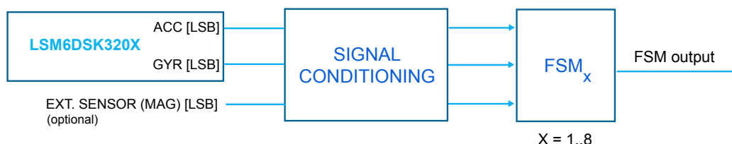
Figure 3. State machine in the LSM6DSK320X
