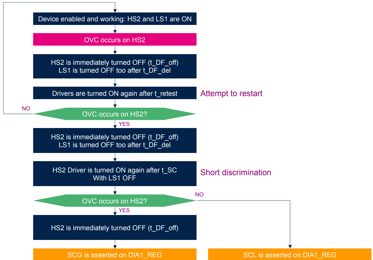
Figure 23. Principle of the short circuit across load detection (OVC on HS2 when PWM = 1)
