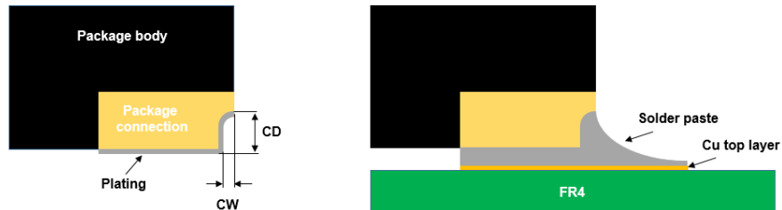
Figure 15. Wettable flank profile
