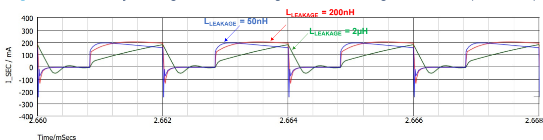
Figure 46. Secondary winding current according to different leakage inductances (simulation)
