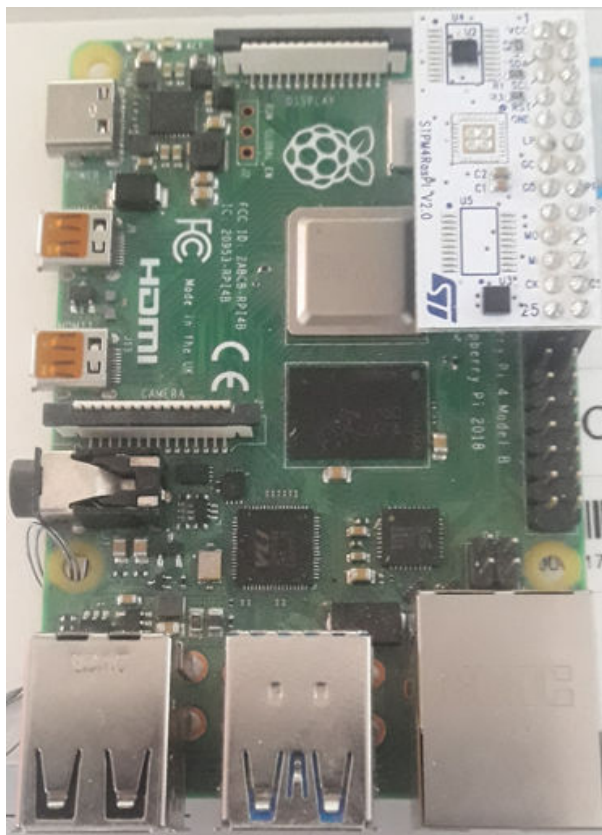
Figure 4. STPM4RasPIV2 with the ST33GTPMISPI and ST33GTPMII2C
