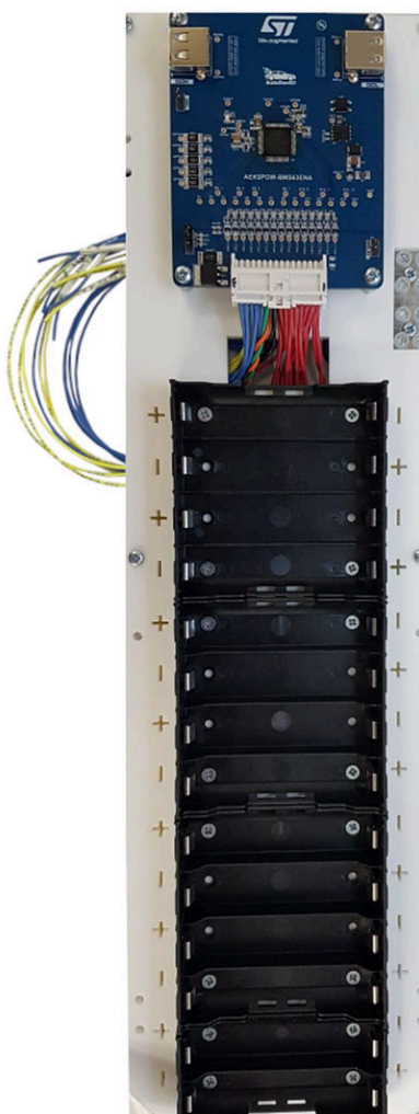
Figure 4. Cables to connect external NTCs
