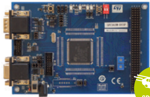
Discovery Kit for the M Line with SPC563M64L7. order code: SPC563M-DISP
