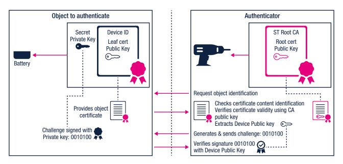
STSAFE-L is a secure element embedded into the object (in this case, the battery) that requires authentication. The secure element contains the battery certificate, which includes a public key and a secret private key. Conversely, the device (a power drill in this example) acts as the authenticator and contains the Certificate Authority (CA) with its public key.
