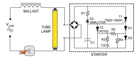
Figure 10. Fluorescent tube starter
