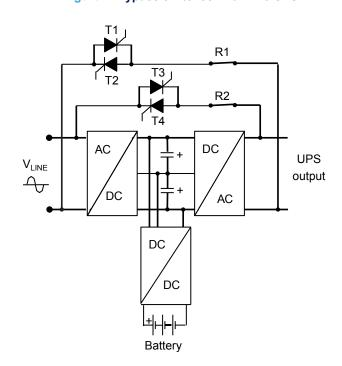
Figure 4. Bypass switches in on-line UPS
