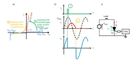
Figure 2. Thyristor static electrical characteristics (a), typical operations (b) and application circuits (c) (b) shows the typical operation of an SCR working in Figure 2. Thyristor static electrical characteristics (a), typical operations (b) and application circuits (c) schematic. The operating sequence is the following:
