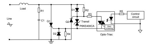
Figure 3. Solid state-relay implemented with two SCRs
