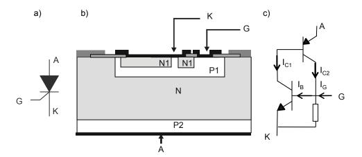
Following its four layer-structure, the thyristor is equivalent to two bipolar transistors interconnected together like shown in Figure 1. Thyristor (SCR) symbol (a), silicon structure (b) and simplified equivalent diagram (c) (c). The gate, for standard SCRs, is then connected to the base of the NPN transistor. This is the reason why a thyristor can only be triggered by a positive gate current (applied from G to K).
