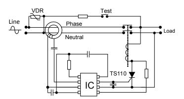
Figure 5. Typical GFCI circuit
