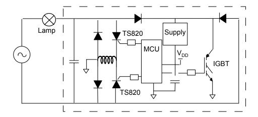
Figure 12. Dimmer for halogen, CFL and LED lamps
