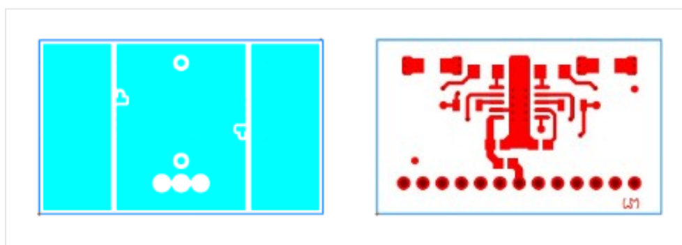
Figure 39. SRK2001A daughterboard layout – top and bottom sides
